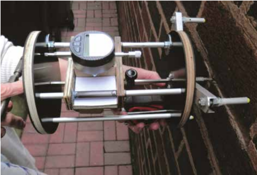
Figure 4: The GFT in-situ mortar tester being used on-site.
