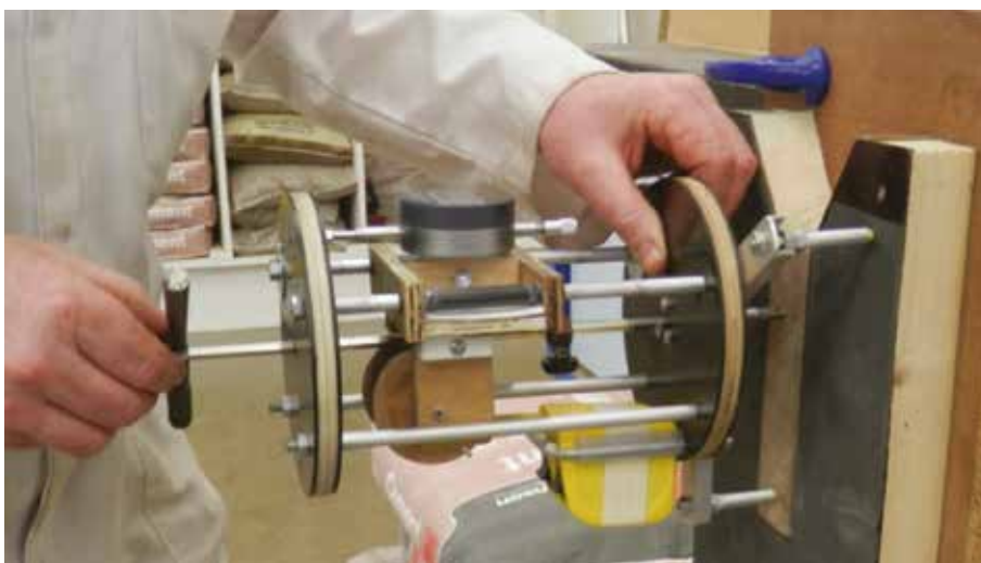
Figure 3: Mark 2 Prototype – GFT in-situ mortar tester under calibration at Wolverhampton University. This machine is fitted with dual constant force springs and can be seen taking readings on a BS mortar test beam.
